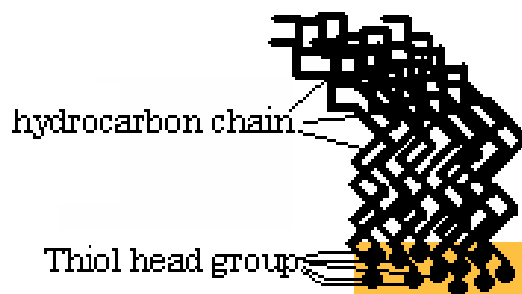
Figure 3: diagram of a SAM on a gold slide
