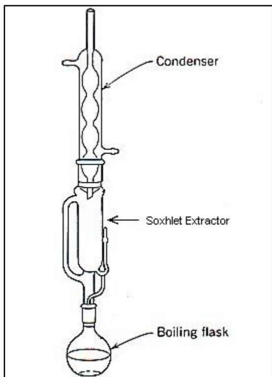
Figure IV-4: Soxhlet extraction apparatus. Organic solvent is vaporized in the boiling flask, and passes through sediment placed in the extraction chamber (middle). A continuous flow of cold water fuels the condenser, in which B[a]P collects and from which solvent drips back down into sediment and the boiling flask.<sup>13</sup>
