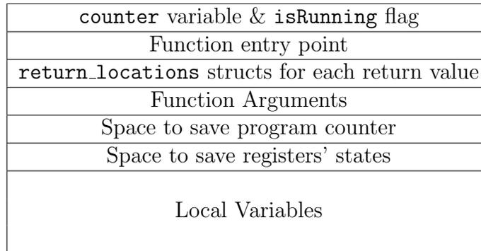
Figure 3.2: This diagram shows the structure of our modified activation records that are stored on the heap. The `counter` variable and `isRunning` flag are stored as one machine word to allow atomic instructions to modify and/or view both in one instruction. See Section 3.1.5.2 for more information.
