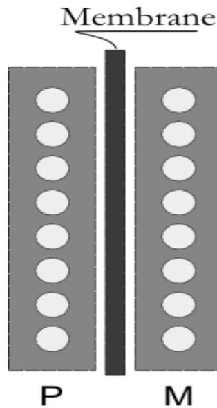
*Figure 5: Schematic of the equilibrium dialysis apparatus*
