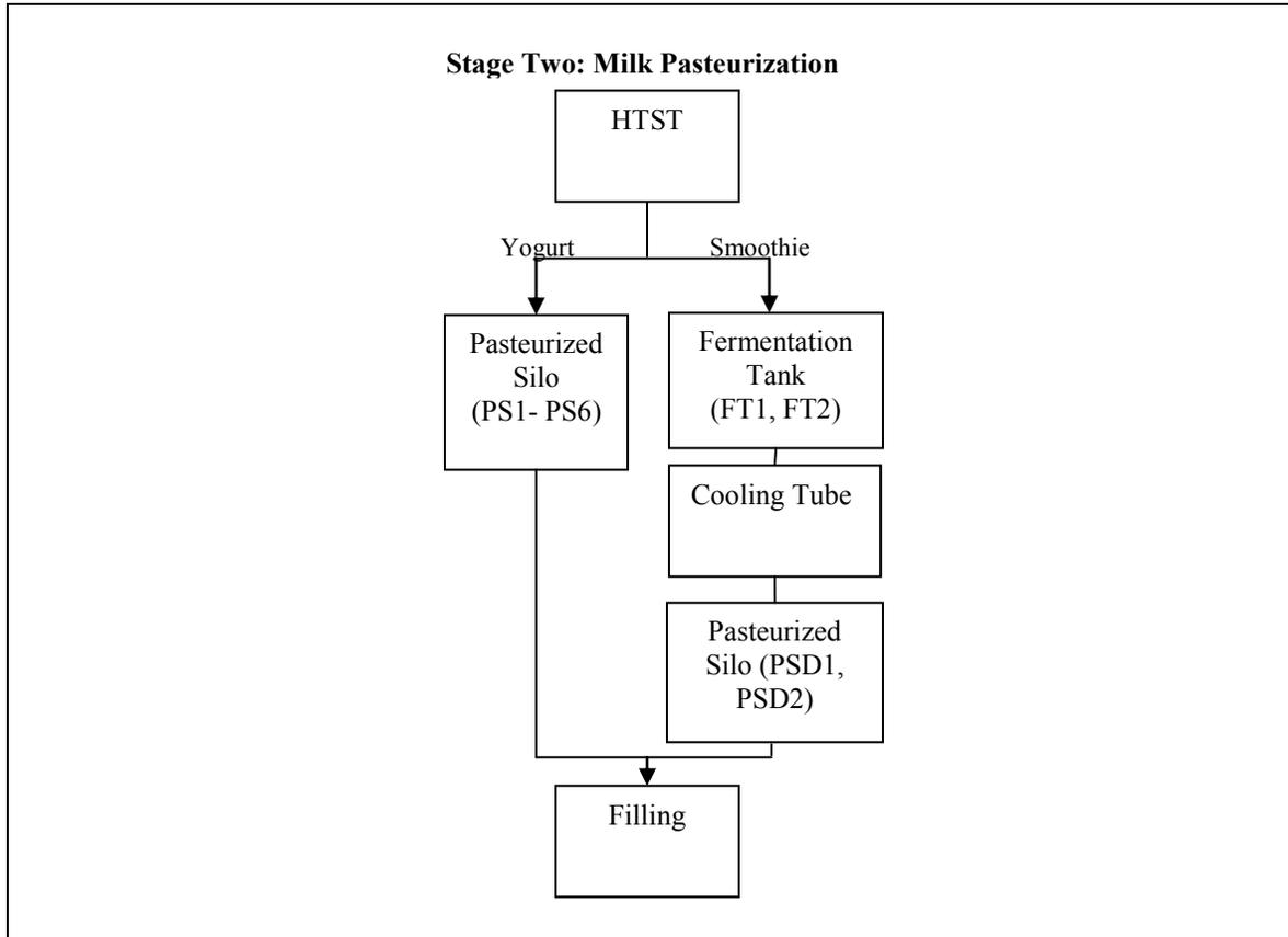
**Figure 4.2 - Process Flow Chart: Milk Pasteurization**
