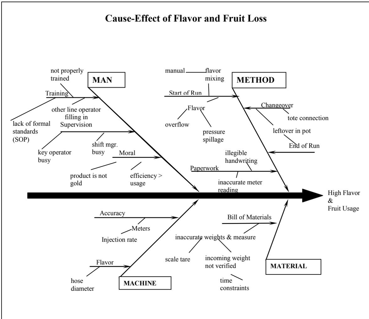
**Figure 4.5 – Fishbone Diagram of Areas of Flavor & Fruit Loss**
