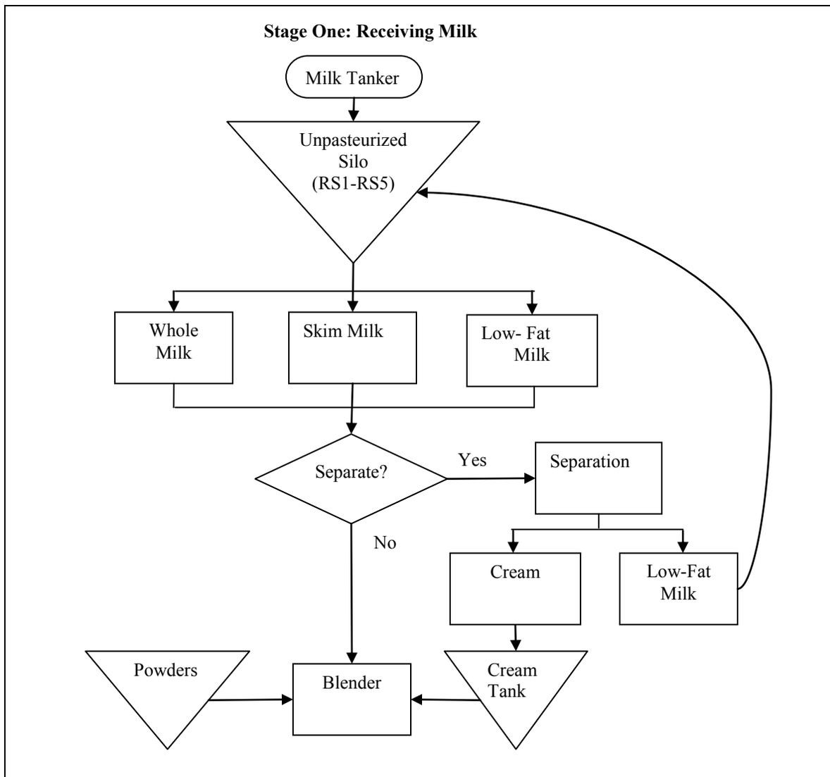
**Figure 4.1 - Process Flow Chart: Receiving Milk**
