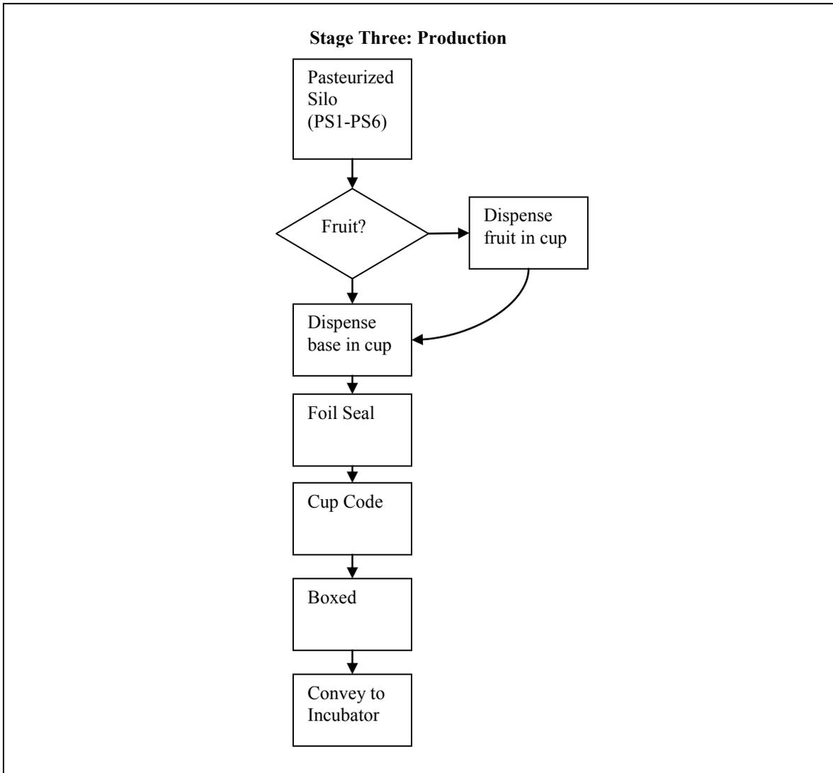
**Figure 4.3 - Process Flow Chart: Production**
