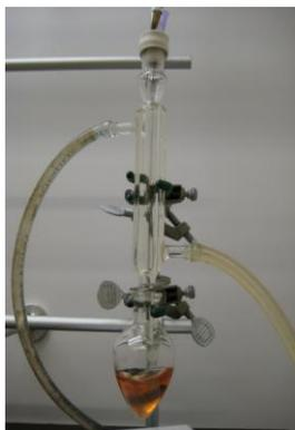
**Figure 9.** Experimental setup for the POSS-ViPy synthesis
