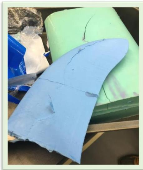
*Figure 8: Final prosthetic flipper removed from mold.*
