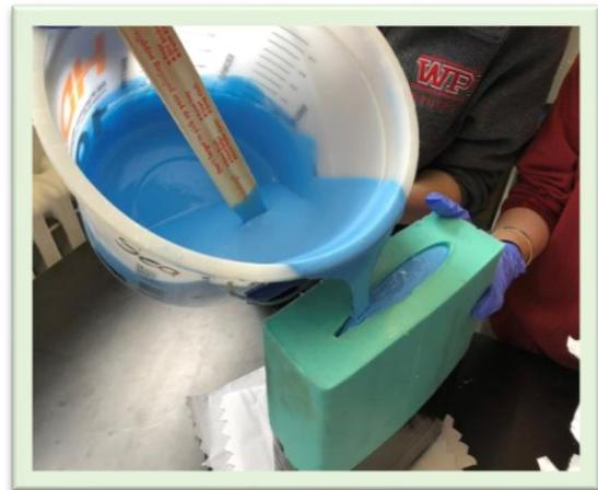
*Figure 7: Pouring the Smooth-Sil 950 into the mold*
