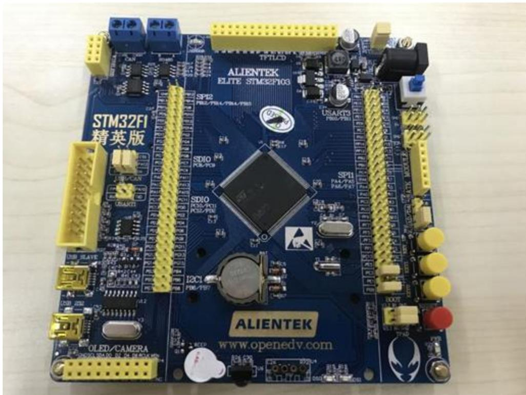
*Figure 10 STM32F103 Integrated Circuit*
