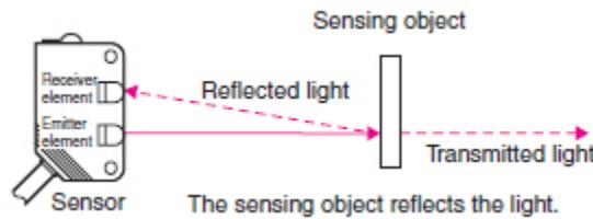
Figure 6 Diffuse-reflective Sensors
