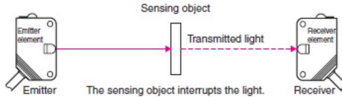
Figure 4 Through-beam Sensors
