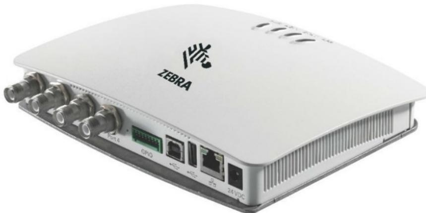
Figure 4: Zebra FX7500 RFID Reader. Taken from [15].
