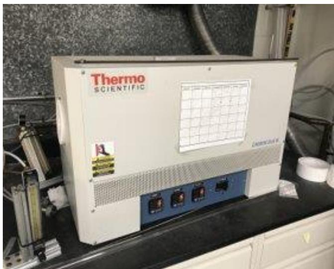
Figure 5: Three-chamber tube furnace
