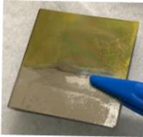
*Figure 7: Indium sulfide film on Mo-coated glass substrate*
