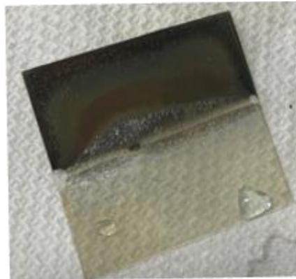
*Figure 8: Indium sulfide on PET flexible substrate*
