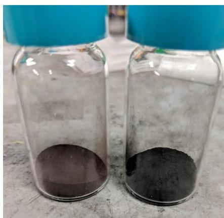
Figure 8: De-lithiated  $\text{Li}_{1-x}\text{Mn}_2\text{O}_4$  Powder (Left) and  $\text{LiMn}_2\text{O}_4$  Powder (Right)
