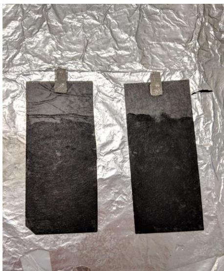
Figure 5: Finished Electrodes with Nickel Foil Attached to the Top
