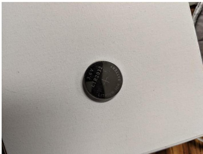
Figure 12: Coin Cell Made with  $\text{LiMn}_2\text{O}_4$  Cathode
