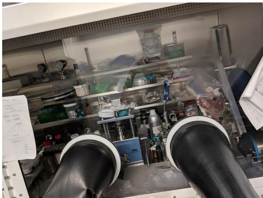
Figure 11: Vacuum Glove Box Used to Create Coin Cells
