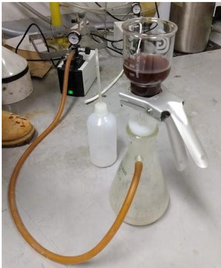
Figure 7: Compression Filter Setup for De-lithiation Process
