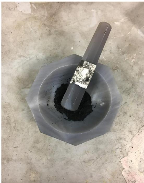
Figure 2: Mixture of  $\text{LiMn}_2\text{O}_4$  and Conductive Carbon Black
