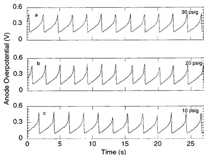
**Figure 9.** Potential oscillation of PEM fuel cell at 42°C at different cathode O<sub>2</sub> pressures: (a) 30, (b) 20, and (c) 10 psig. Current density 300 mA/cm<sup>2</sup>; anode inlet flow rate 48.1 sccm.
