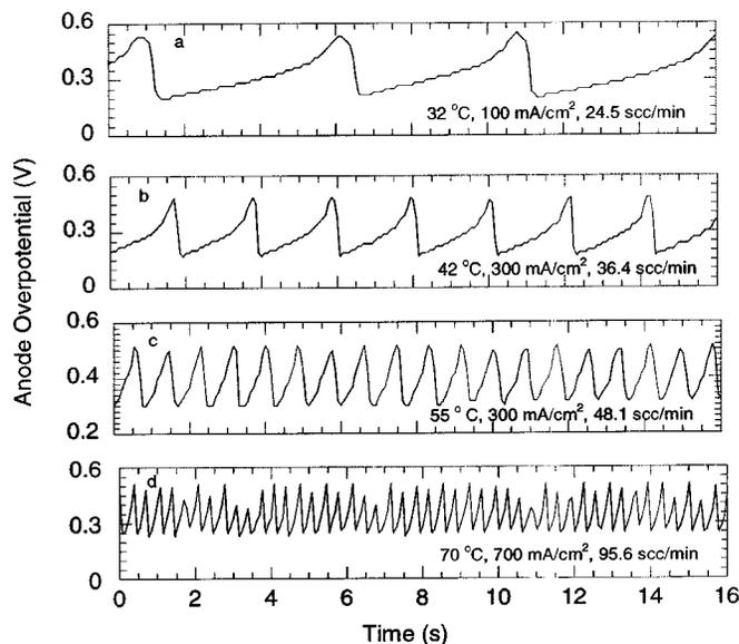
**Figure 7.** Potential oscillation of PEM fuel cell at different temperatures. The fuel-cell temperature, applied current density, and anode inlet flow rate are, as follows: (a) 32°C, 100 mA/cm<sup>2</sup>, 24.5 scc/min; (b) 42°C, 300 mA/cm<sup>2</sup>, 36.4 scc/min; (c) 55°C, 300 mA/cm<sup>2</sup>, 48.1 scc/min; and (d) 70°C, 700 mA/cm<sup>2</sup>, 95.6 scc/min.
