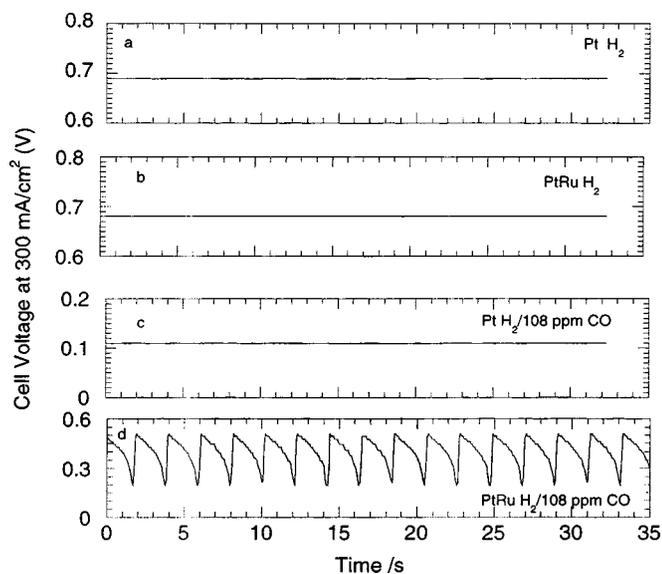
**Figure 1.** Fuel-cell voltage pattern for (a) Pt with H<sub>2</sub>, (b) PtRu with H<sub>2</sub>, (c) Pt with H<sub>2</sub>/108 ppm CO, and (d) PtRu with H<sub>2</sub>/108 ppm CO. Other operation conditions are identical: cell temperature 42°C; current density 300 mA/cm<sup>2</sup>; anode inlet flow rate 36.4 sccm.
