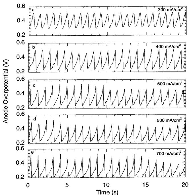
**Figure 4.** Potential oscillation of PEM fuel cell at 55°C at different current densities: (a) 300, (b) 400, (c) 500, (d) 600, and (e) 700 mA/cm<sup>2</sup>. Anode flow rate is 48.1 sccm for all cases.
