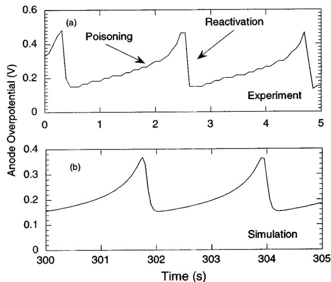
**Figure 8.** A magnified picture of the potential oscillation pattern from (a) experiment and (b) simulation at 42°C. Current density 300 mA/cm<sup>2</sup>; anode inlet flow rate 48.1 scc/min.
