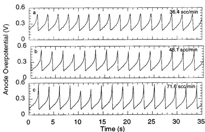
**Figure 5.** Potential oscillation of PEM fuel cell at 42°C at different anode inlet flow rates: (a) 36.4, (b) 48.1 and (c) 71.6 sccm. The current density is 300 mA/cm<sup>2</sup> for all cases.
