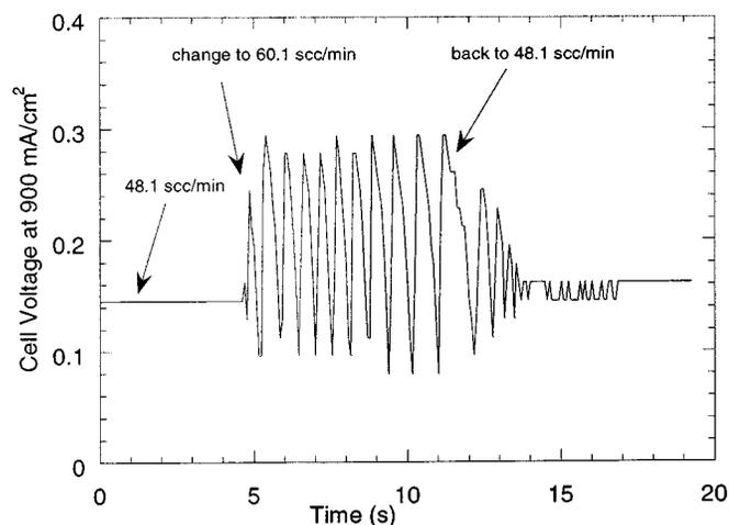
**Figure 3.** The transition of the fuel-cell voltage between a steady value and oscillation with the variation of anode flow rate. Cell temperature 70°C; current density 900 mA/cm<sup>2</sup>.
