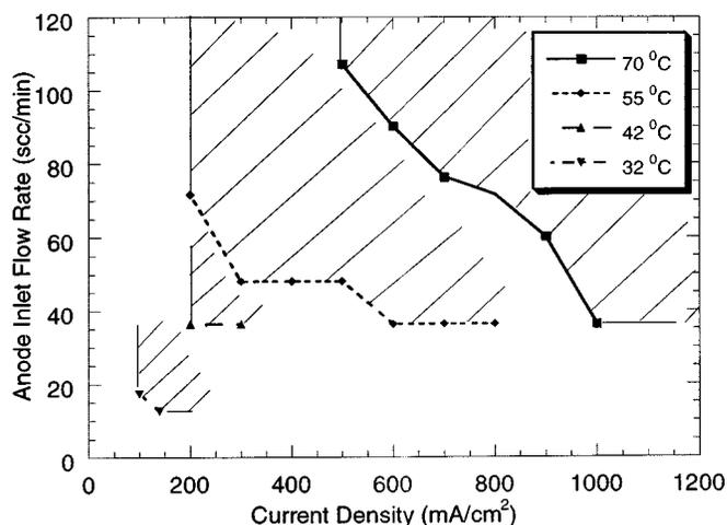
**Figure 2.** The current density-anode flow rate domain where anode overpotential oscillation appears at different temperatures.
