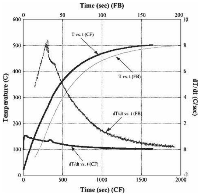
Fig. 13—Thermal analysis of 319 type alloy during solution heat treatment using a CF and an FB.
