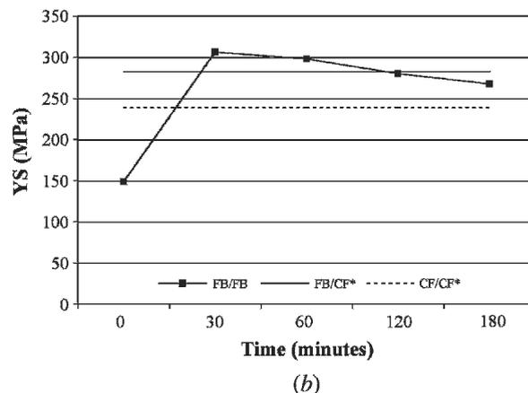
Fig. 17—Effect of aging 354 alloy at 200 °C on (a) UTS and elongation (E) and (b) YS. Note: FB/FB: FB solutionized and FB aged; FB/CF\*: FB solutionized and CF aged; and CF/CF\*: CF solutionized and CF aged. Aging time for FB/CF\* and CF/CF\* is 5 hours.
