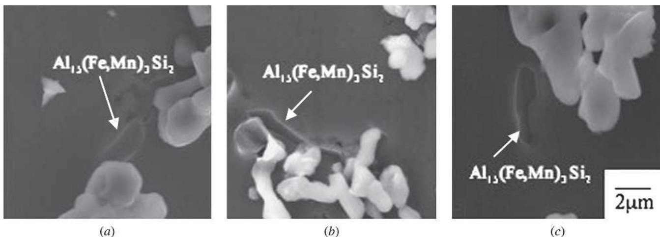
Fig. 8—Effect of the solution heat treatment of 319 alloy using an FB reactor at 493 °C on the morphology of  $\text{Al}_{13}(\text{Fe,Mn})_3\text{Si}_2$  particles for (a) 30 min, (b) 60 min, and (c) 120 min.
