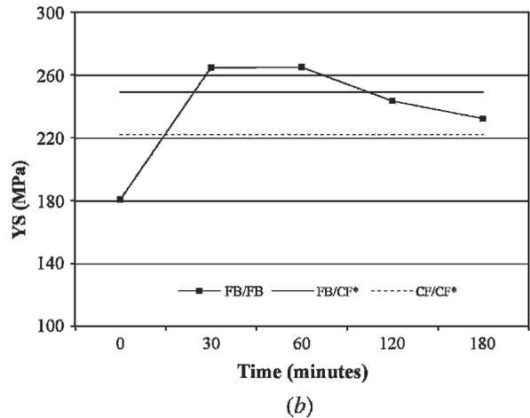
Fig. 19—Effect of aging 319 alloy at 200 °C on (a) UTS and elongation (E) and (b) YS. Note: FB/FB: FB solutionized and FB aged; FB/CF\*: FB solutionized and CF aged; and CF/CF\*: CF solutionized and CF aged. Aging time for FB/CF\* and CF/CF\* is 5 h.
