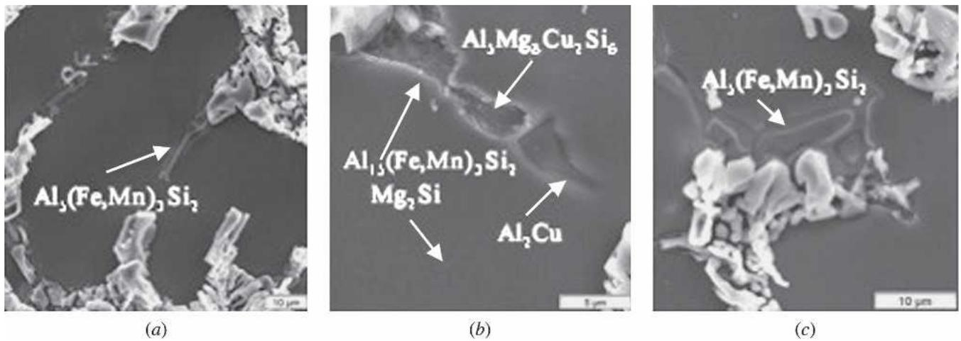
Fig. 5—SEM micrograph of as-cast 319 alloy: (a) eutectic Si; (b) intermetallics such as  $Mg_2Si$ ,  $Al_2Cu$ ,  $Al_{15}(Fe,Mn)_3Si_2$ , and  $Al_3Mg_3Cu_7Si_6$ ; and (c) Fe-rich phase.
