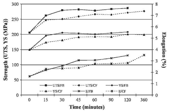
Fig. 15—Variation in UTS, YS, and elongation (E) of 354 alloy solutionized at 527 °C.
