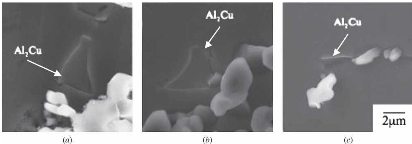
Fig. 7—Effect of the solution heat treatment of 319 alloy using an FB reactor at 493 °C on the morphology of  $\text{Al}_7\text{Cu}$  particles for (a) 30 min, (b) 60 min, and (c) 120 min.
