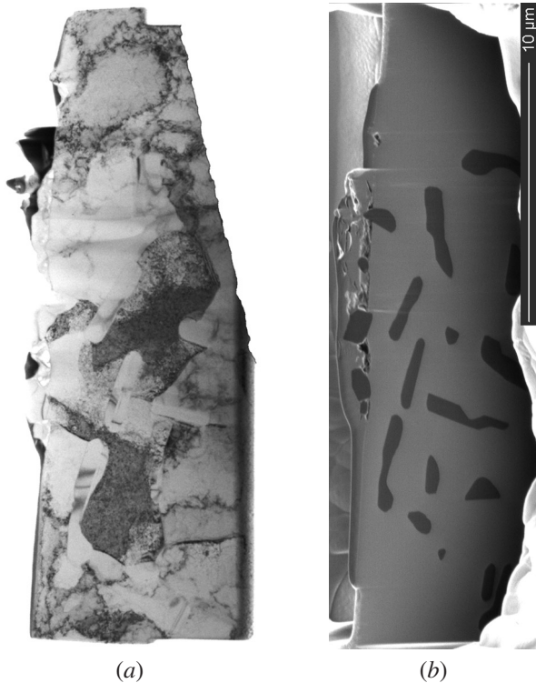
Fig. 3—Comparison of TEM and SEM micrographs of Al-7 pct Si at the desired sample location: (a) low-magnification TEM image of the Al-7 pct Si sample and (b) high-magnification SEM image of the Al-7 pct Si sample.
