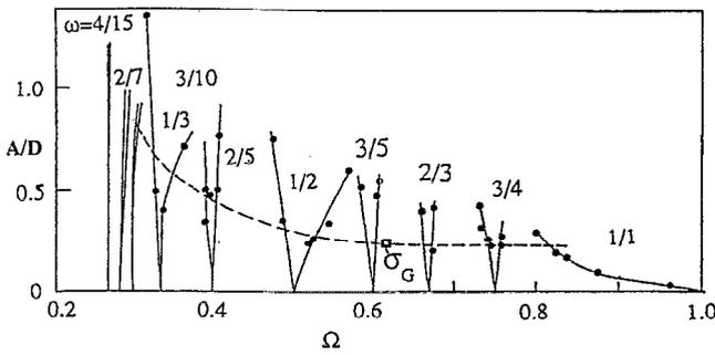
FIG. 4. The experiment  $A/D$ - $\Omega$  plane for the oscillating cylinder-wake system. The regions labeled with  $p/q$  values are lock-in tongues. About 30 such tongues were observed in experiments, but only those with appreciable widths are shown. The critical line for transition to chaos is shown dashed. Reproduced from Ref. 1.
