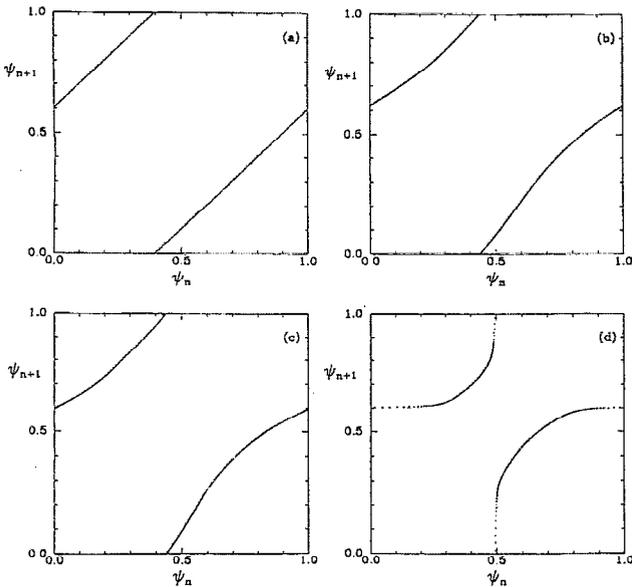
FIG. 5. Return maps from the numerical solution as forcing amplitude  $F'$  is increased.  $\Omega=0.623$ . (a)  $F'=0$ , (b)  $F'=0.1$ , (c)  $F'=0.15$ , and (d)  $F'=0.22$  approximating the critical transition to chaos. Note the appearance of a cubic inflection point with zero slope at  $\psi_n=0$  in (d).
