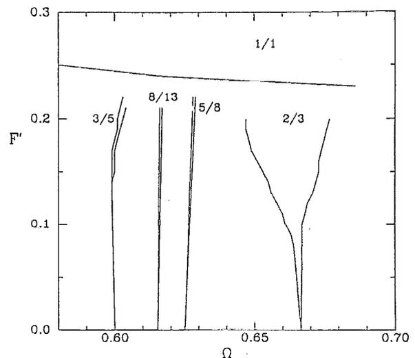
FIG. 3. A portion of the  $F'$ - $\Omega$  plane from the numerical solution. Arnold tongues where lock-in states occur are shown. The tongues widen in extent as the level of forcing  $F'$  increases. Only tongues of significant extent are shown.
