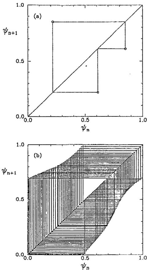
FIG. 1. Return maps for a lock-in and quasiperiodic state from the numerical solution of the forced Landau-Stuart equation. (a) The periodic trajectory of a  $2/3$  lock-in state.  $\Omega=0.648$ ,  $F'=0.2$ ,  $C=1.1$ . (b) The nonrepeating trajectory of a quasiperiodic state.  $\Omega=0.644$ ,  $F'=0.2$ ,  $C=1.1$ .
