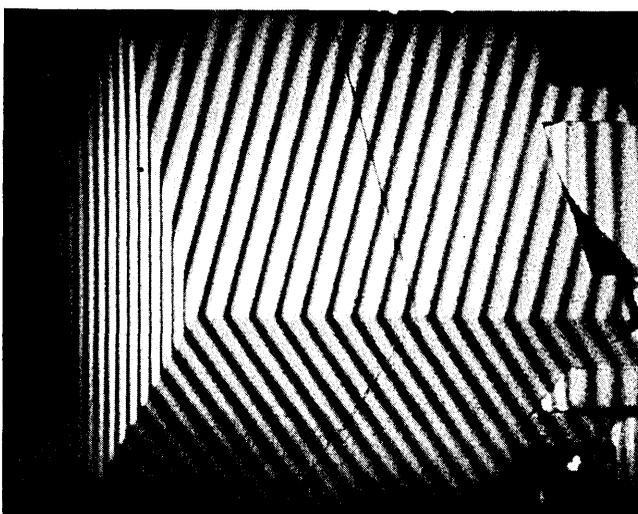
Fig. 2. Reconstruction from a typical double-exposure hologram recording rigid-body rotation of an object.
