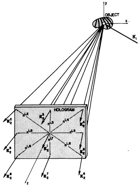
Fig. 3. Schematic representation of multiple observations of a holographic image.  $\mathbf{K}_1$  is the illumination vector;  $\mathbf{K}_2^1, \mathbf{K}_2^2, \dots, \mathbf{K}_2^r$  are observation vectors.
