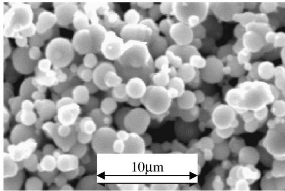
FIG. 1. SEM image of carbonyl iron particles.
